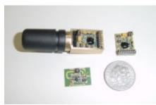
TJ1004 is TChip's single chip L1 C/A GPS receivers. Innovative design techniques, give the TJ1004 the industry's lowest power consumption (<5mA fully active!) Combined with a minimum number of external components this enables a supersmall receiver for handheld applications. For
