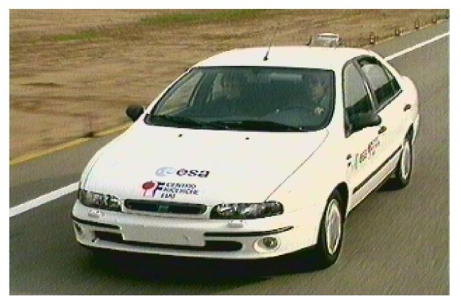
An EGNOS receiver was installed in a FIAT car and linked to a PC running digital mapping software
